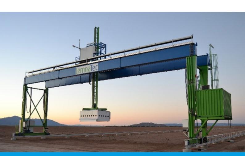
The FieldAlxpert can be equipped with the full range of imaging systems for structural and physiological phenotyping of the growing vegetation. Thereby it enables continuous phenotypic analyses of the developing crops.
